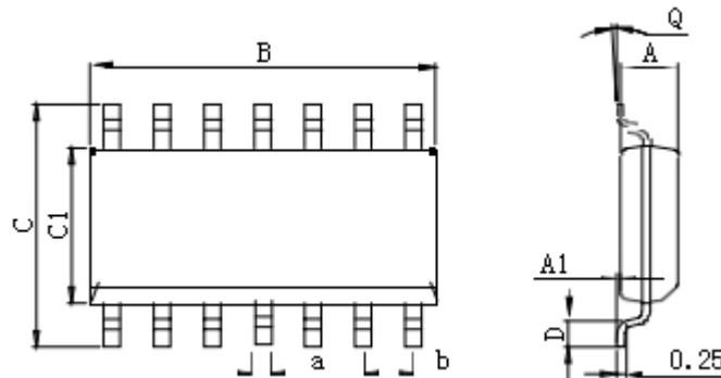
Dimensions In Millimeters(SOP14)
