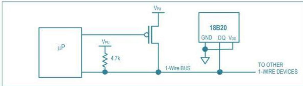
图 5. Powering the 18 B 2 0 with an External Supply
